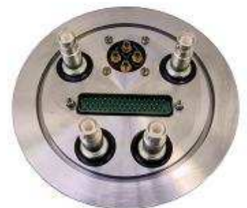
ISO K DN100 Equipped with 4 x 14kV Reynolds 4 x 3.5kV SHV 1 ERVAC50M/F-I-ND
